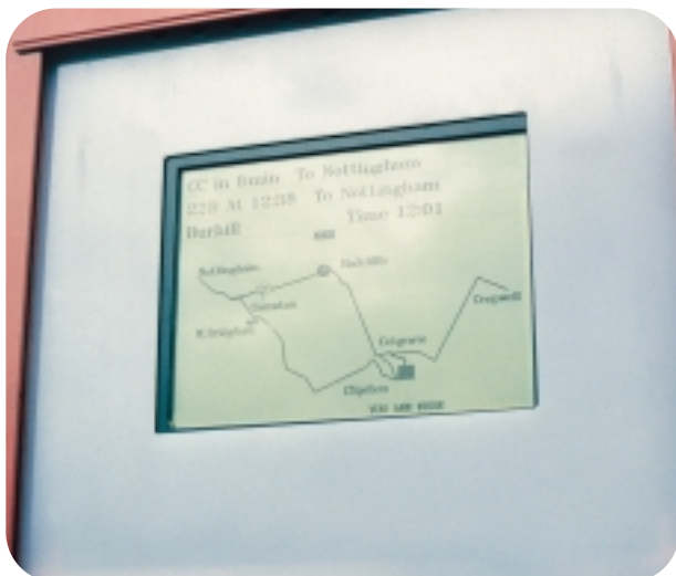
LCD map style display fits into an infopole layout and was first used on the "Cotgrave Connection" service, a Quality Partnership initiative with Barton and Nottinghamshire CC. Photo: Trent-Barton Buses/Nottingham County Council.
