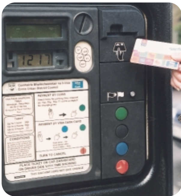
SchlumbergerSema P&D terminals in Ennis, Ireland have been upgraded to accept Visa Cash smart cards, as well as cash.
